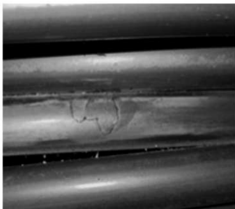
图 1 10B21 钢线材表面结疤形貌 Fig. 1 Morphology of scarred surface of 10B21 steel wire
